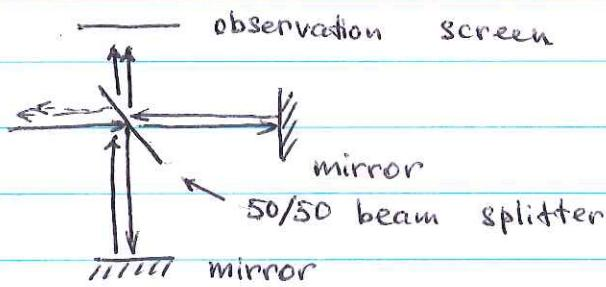
If one of the mirrors moves by  $\lambda/2$ , the interference switches from constructive to destructive
