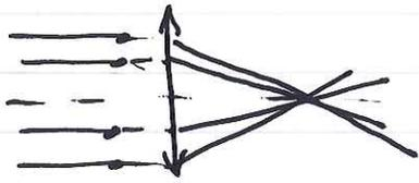
Ideal lens changes the beam direction without any displacements independently on where the beam hits the lens.
