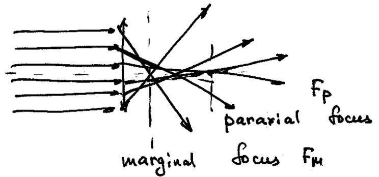
The larger is the distance b/w  $F_p$  and  $F_m$ , the larger is spherical aberration.
