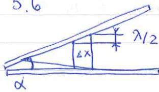
The distance in thickness b/w two bright (or dark) lines is  $\lambda/2$  (since the reflected beam travels this thickness of the slab twice)
