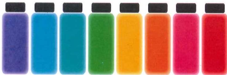
Depending on size, quantum dots emit different color light due to quantum confinement. Illustrated is the range of QDs with emission gradually stepping from violet to red.
