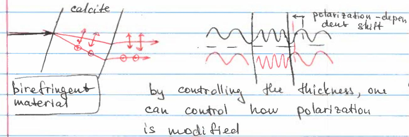
Liquid crystals are strongly birefringent, and the refractive index difference depends on applied voltage, so one can control the output polarization by applying voltage.
