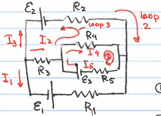
$$\left. \begin{array}{l} I_1 + I_2 + I_3 = 0 \\ I_2 = I_4 + I_5 \end{array} \right\} \text{current rules}$$
