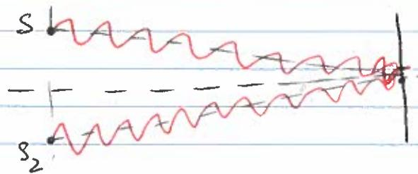
The center is equidistant from the two sources, two arriving waves are identical \$\rightarrow\$ constructive interference
