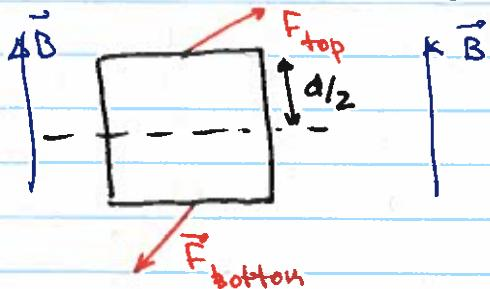
Each force tries to rotate the loop in the same direction
