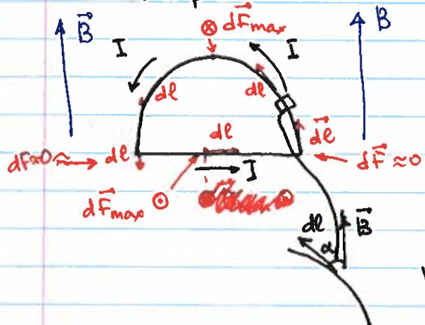
The magnetic force per unit length is strongest in the straight part and on top
