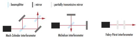
**Mach–Zehnder** interferometers utilize one beamsplitter to separate an input beam into two separate paths. A second beamsplitter recombines the two paths into two outputs, which are sent to photodetectors. **Michelson interferometers** use a single beamsplitter for splitting and recombining the beams. **Fabry–Perot** interferometers allow for multiple trips of light by using two parallel partially transparent mirrors instead of two separated beam paths.
