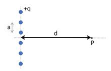
Our goal is to determine the electric field in point P, which is positioned at distant d from the charge line and passes through its center (i.e., it is the symmetry line for any charge configuration).
