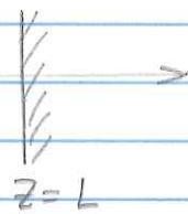
$$\begin{aligned} \epsilon &= 1 & \mu &= 1 \\ \vec{E}(z=0) &= \vec{E}(z=L) = 0 & \text{boundary conditions} \end{aligned}$$
