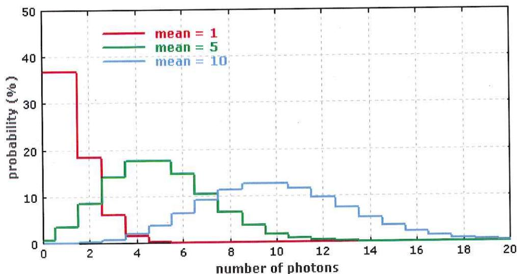
Photon distribution in coherent states with different mean value of photon  $|d\rangle$
