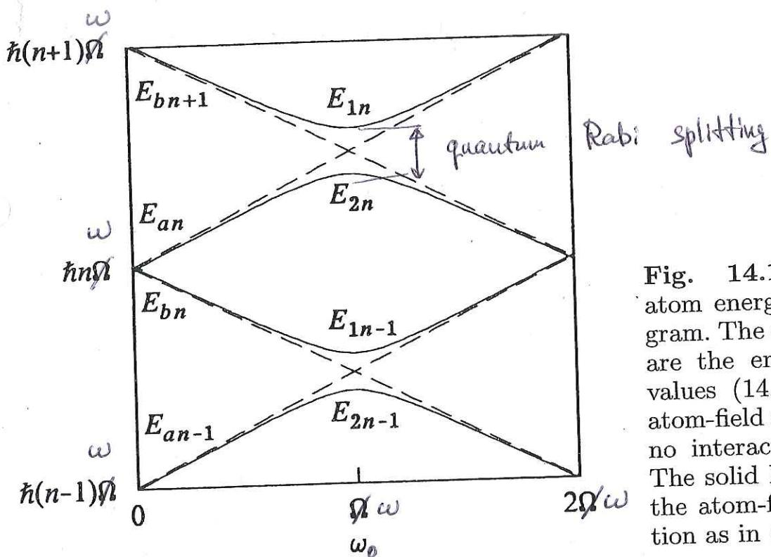
**Fig. 14.1.** Dressed atom energy level diagram. The dashed lines are the energy eigenvalues (14.11) for the atom-field system with no interaction energy. The solid lines include the atom-field interaction as in (14.14)
