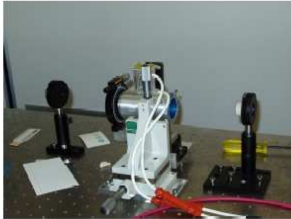
FIG. 3.4: A Pockels Cell between two linear polarizers.
