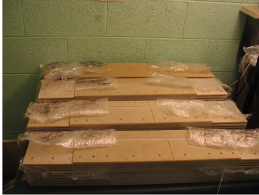
Figure 3.3: This photo illustrates the 4 different components that the G10 frames were constructed out of. These four components were epoxied and clamped together to create the G10 frame.
