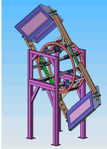
Figure 2.5: Chambers are placed at opposing octants so that two measurements can be made at a time. A total of 4 measurements will need to be made in order to cover the entire detector system.
