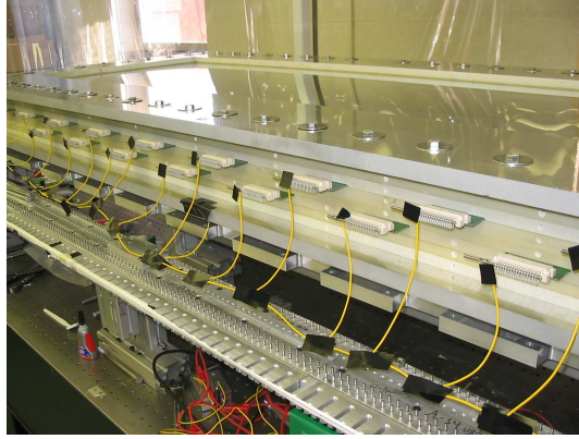
Figure 4.2: This figure illustrates how the readout cards and therefore the sense wires were grounded while applying high voltage to the drift chamber. Small aluminum rods were soldered to each DIN pin connector and then wires were soldered to each of the aluminum rods. The aluminum rods were connected to one another using a grounding wire. The end of the grounding wire was then taped on to the aluminum frame to ensure a ground connection.
