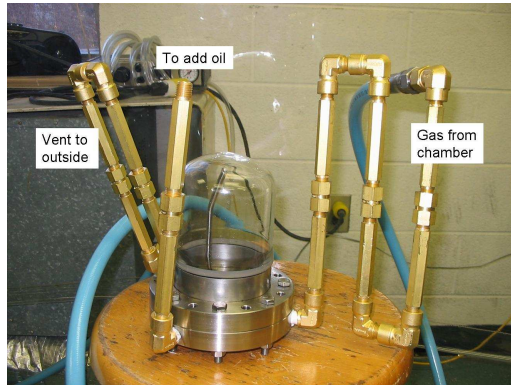
Figure 3.10: This photo shows the bubbler that was constructed for the gas handling system. Gas from the chamber enters the bubbler and then “bubbles” through a thin layer of mineral oil. Since the gas can not penetrate the mineral oil, it is vented out through another tube due to the pressure that builds up inside.
