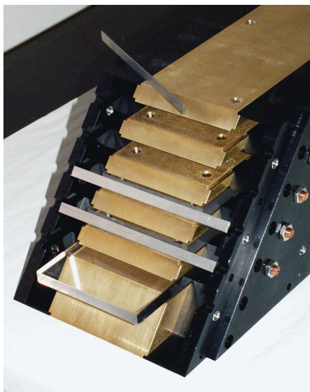
FIG. 2.19: Cutaway view of the HAPPEX detector quartz and brass layers.
